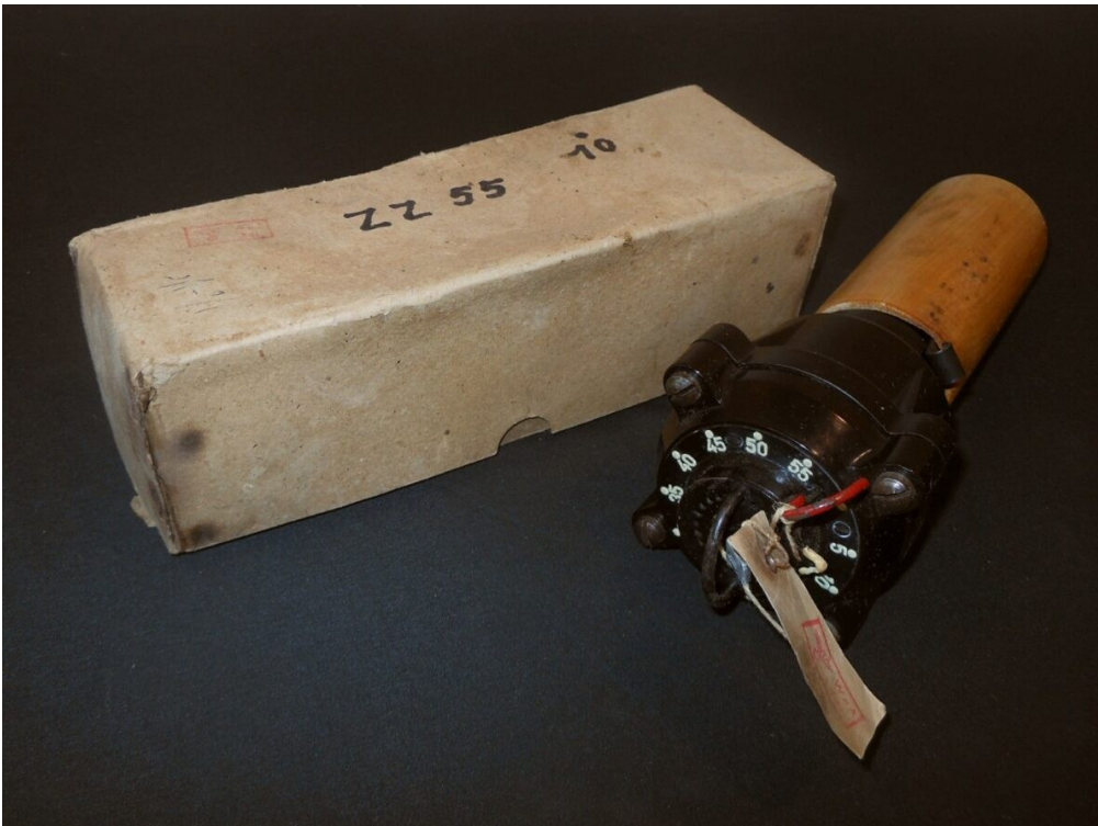
Zt.Z. 55 Firing Device with wooden sleeve and packing box.
