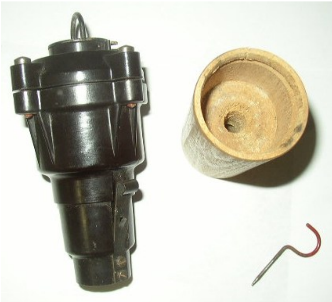
Zt.Z. 55 Firing Device with wooden sleeve and arming pin
