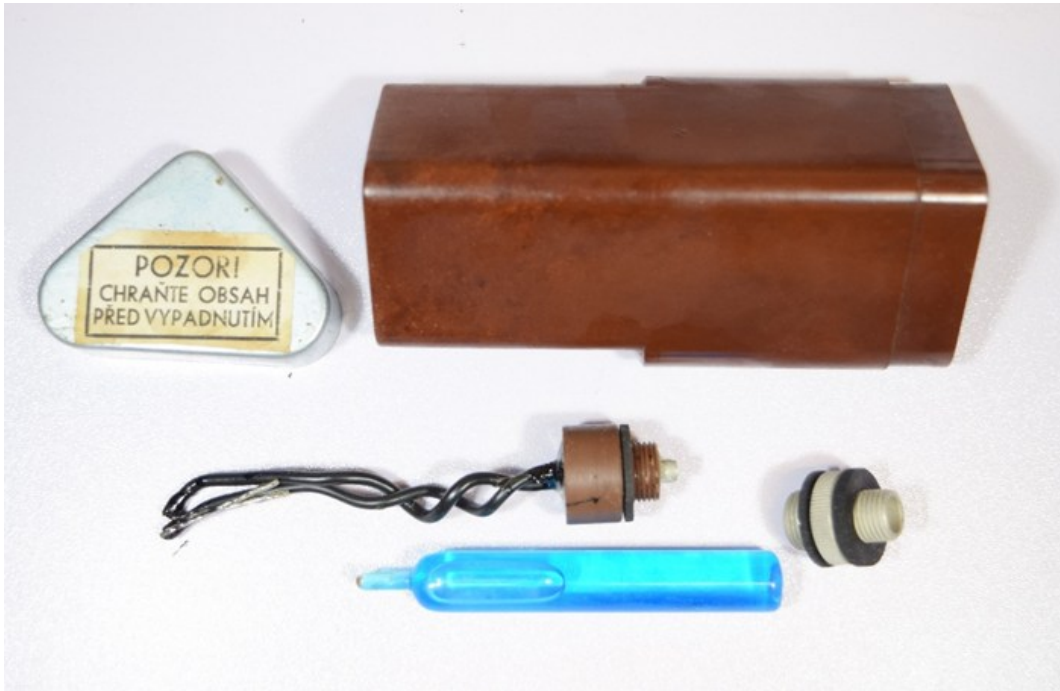
ECHRO accessory pack containing electrical initiation, mechanical initiation and chemical components Photo - G. Zahaczewsky
