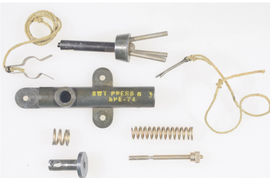
No. 5 Firing Device (disassembled) (Note the broken threads on the extension rod) Photo - G. Zahaczewsky
