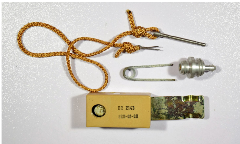
NR 2143 Firing Device (disassembled) Photo - G. Zahaczewsky
