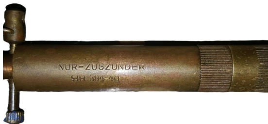
Zu.Z.Z. 35 Firing Device Modified markings
