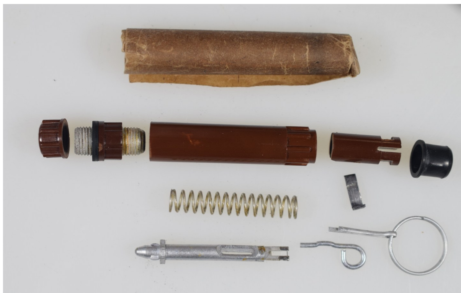
MUV - 2M Firing Device (disassembled) Photo - G. Zahaczewsky
