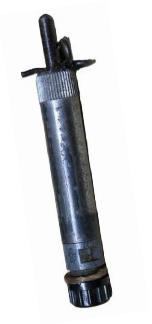
Zu.Z.Z. 42 Firing Device (steel body)
