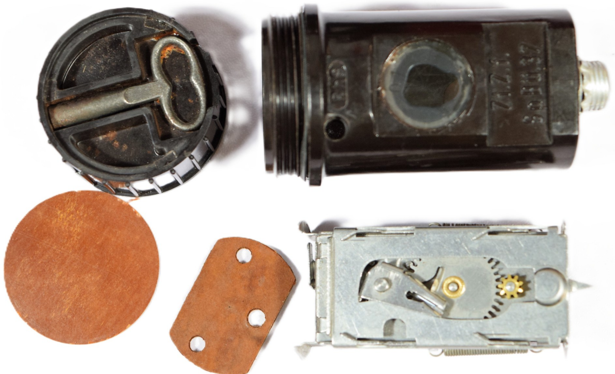
Zt.Z.f.SpBü 37 Firing Device components - Type II Photo - G. Zahaczewsky
