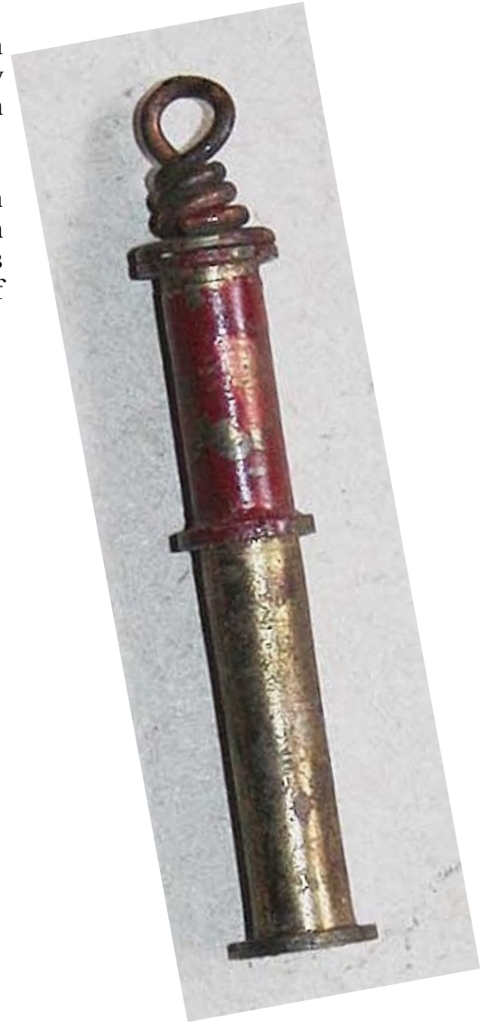
Friction Fuse Igniter Model 13
