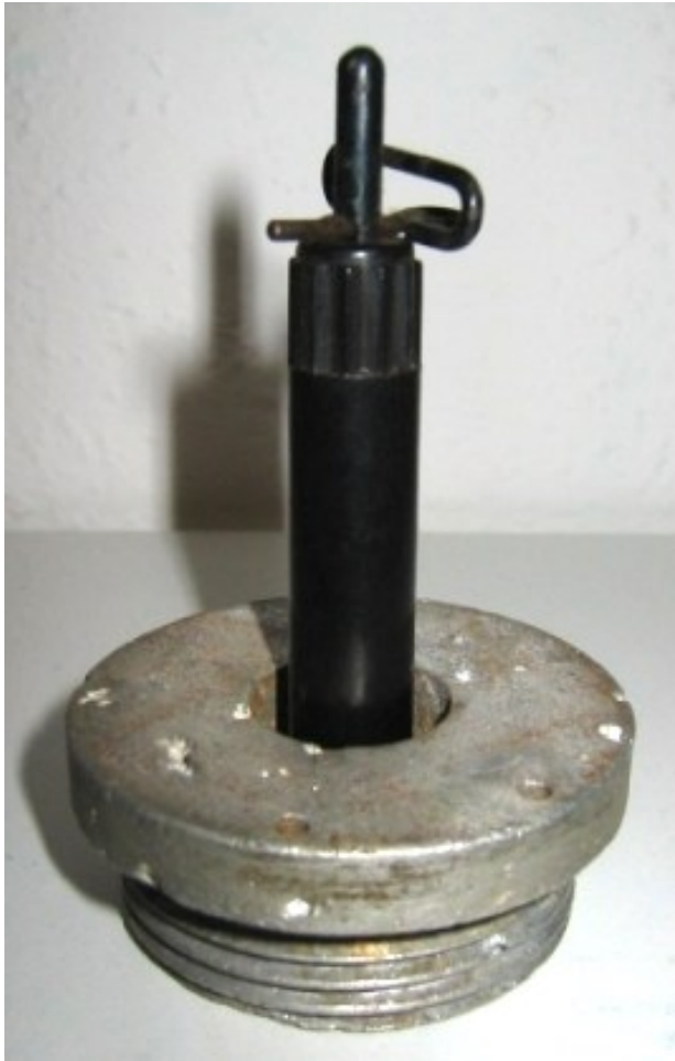
Aluminum adapter fitted with Z.Z.42
