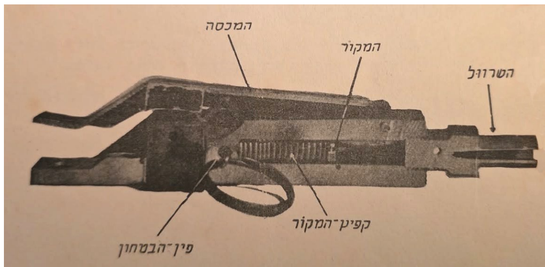
Release mechanism 104 internal diagram (From Israeli manual)
