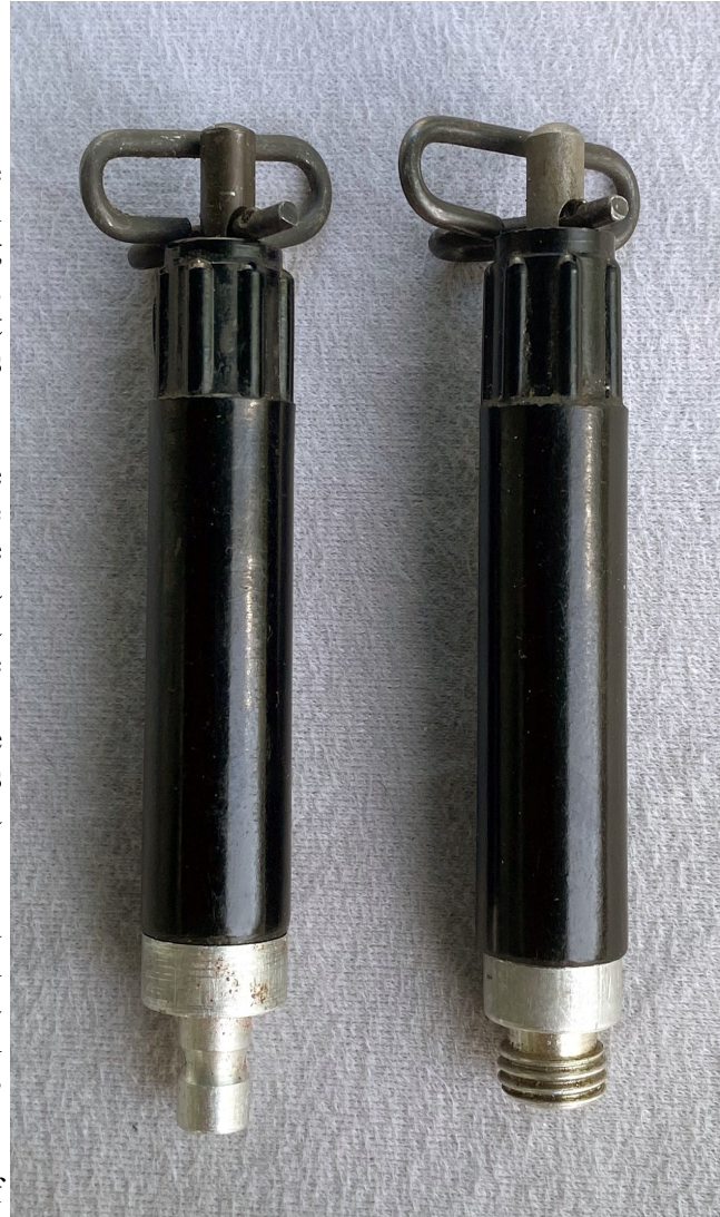
Ro 1 Firing Device East German Copy (Note the difference in the primer holders)
