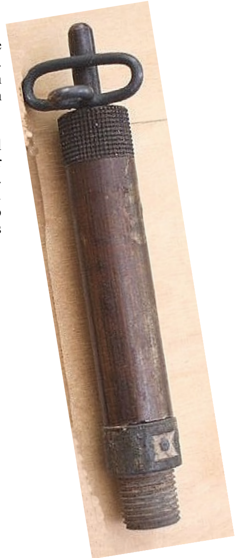
Zu.Z.Z. 42 Firing Device (Norwegian production)
