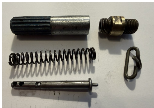
M/47 Firing Device (disassembled) Photo - G. Zahaczewsky
