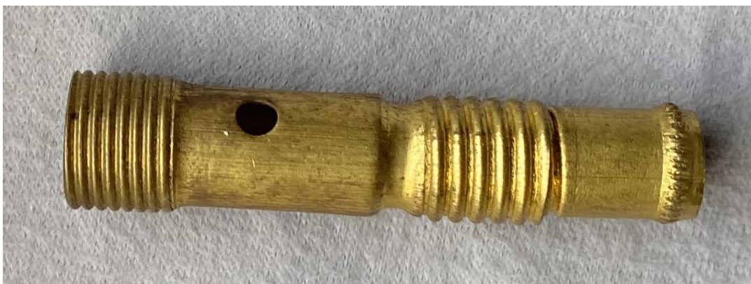
Connection sleeve and collet Klemmhülse and Verbindungs
