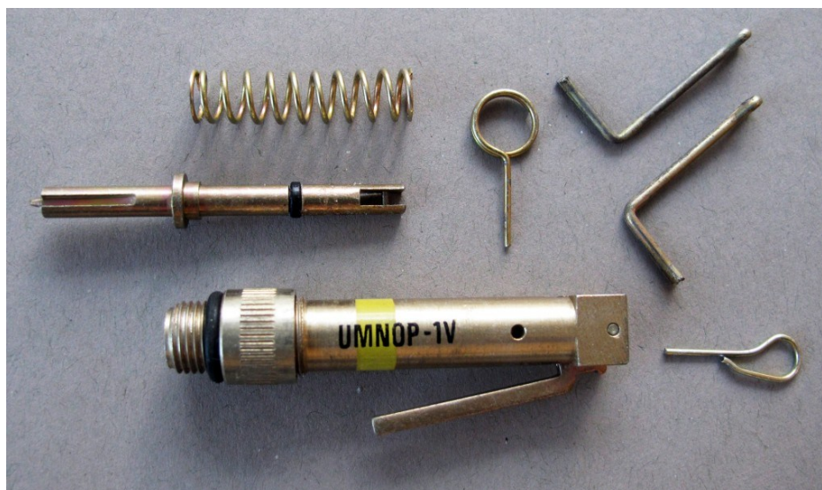
UMNOP-1V Practice Firing Device (partially disassembled revealing the striker), Photo – Fenix Insight
