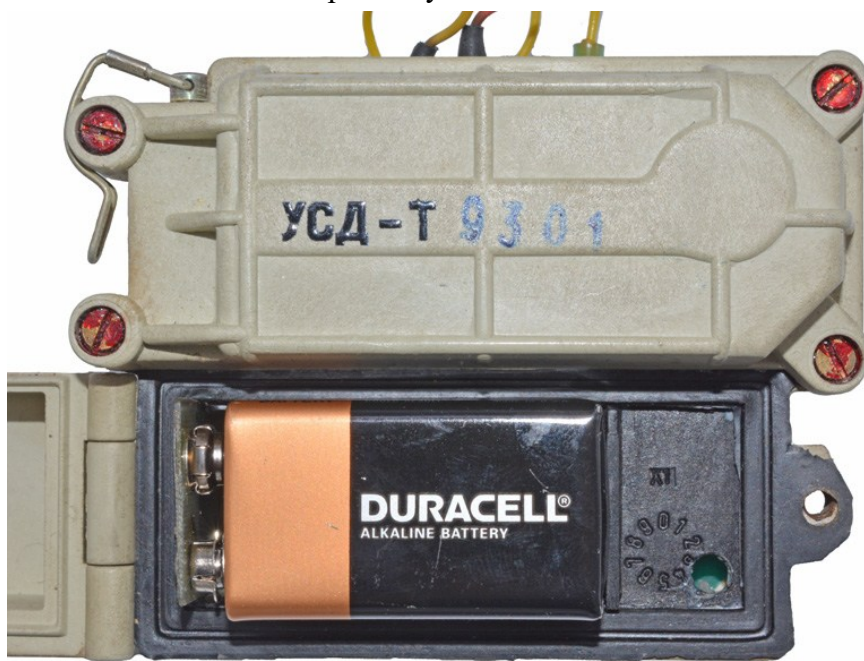
USD-T battery compartment Photo- Bob Leiendecker
