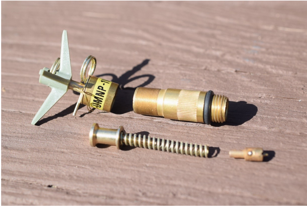
UMNP-1V Training Device (disassembled) Image – G. Zahaczewsky
