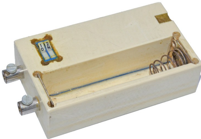
U-TE Firing Device (bottom view showing battery compartment) Photo – Bob Leindecker
