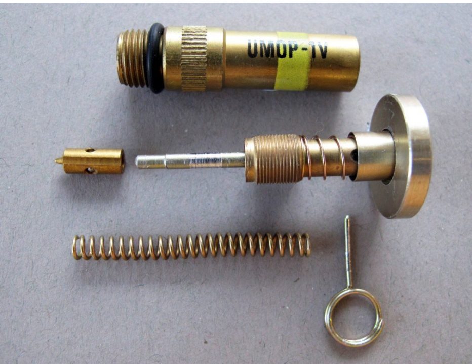
UMOP-1V Practice Firing Device (disassembled) Photo – Fenix Insight
