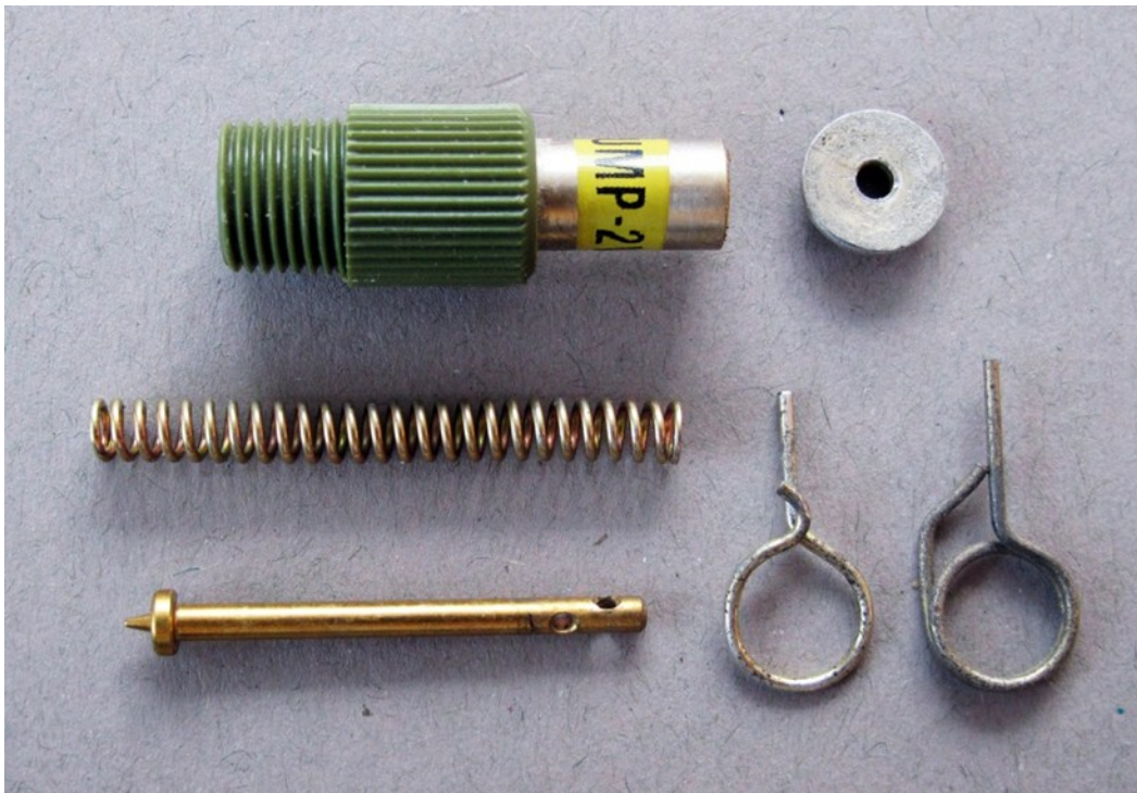
UMP-2V Practice Firing Device (disassembled) Image – Fenix Insight
