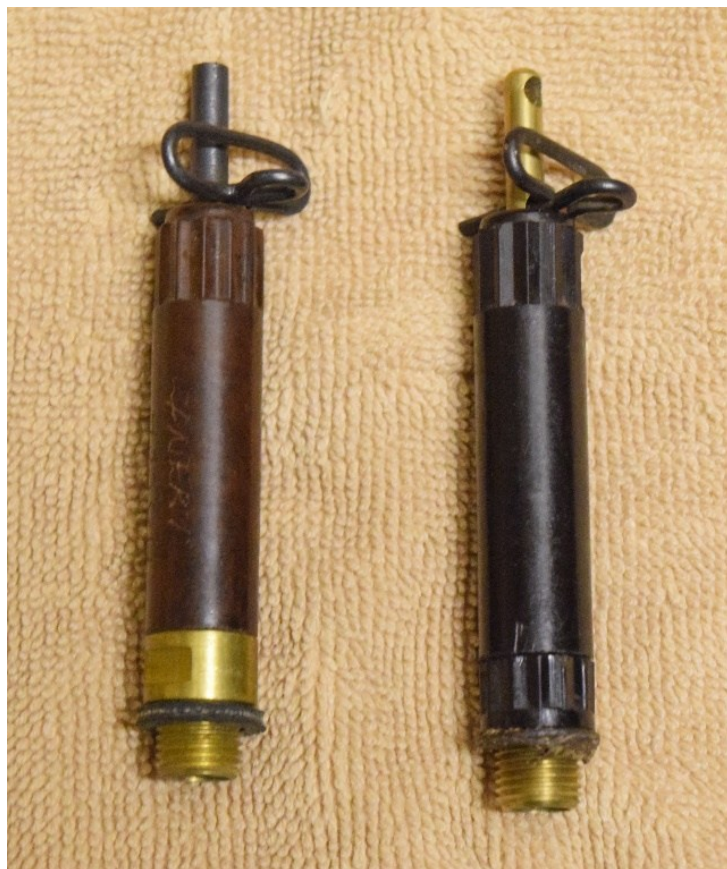
Yugoslav UPM-1 (left) and German Z.Z.42 (right) Firing Devices Photo – G. Zahaczewsky
