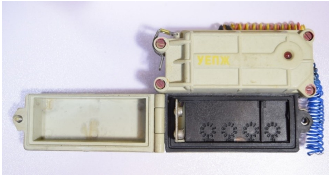
UEPZh microswitch delay arming mechanism (which is found in all “super quick fuzes” NOTE Honeywell markings) Photo – G. Zahaczewsky
