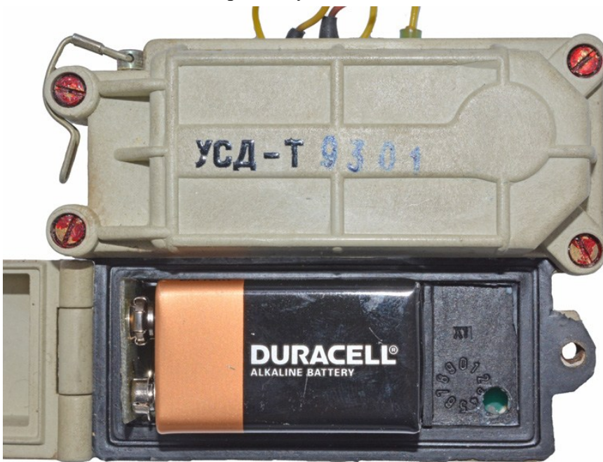
USD-T battery compartment Photo- Bob Leiendecker
