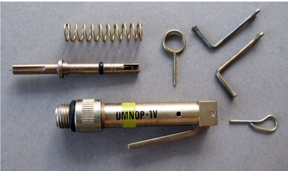
UMNOP-1V Practice Firing Device (partially disassembled revealing the striker), Photo – Fenix Insight
