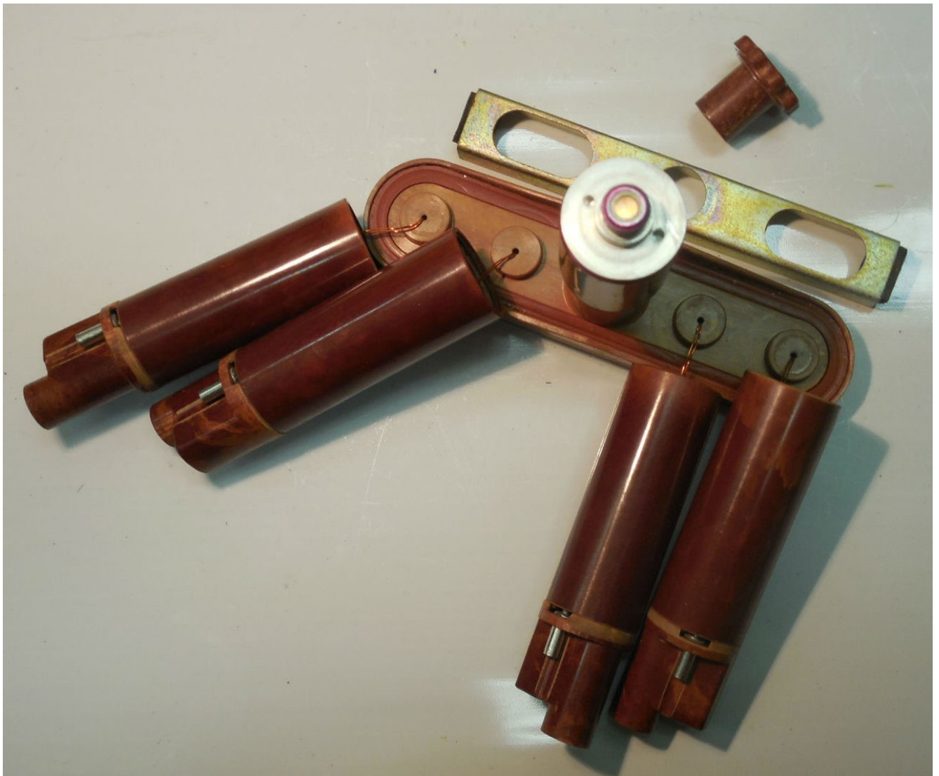
VUZ-4 Firing Device showing the ignition assemblies
