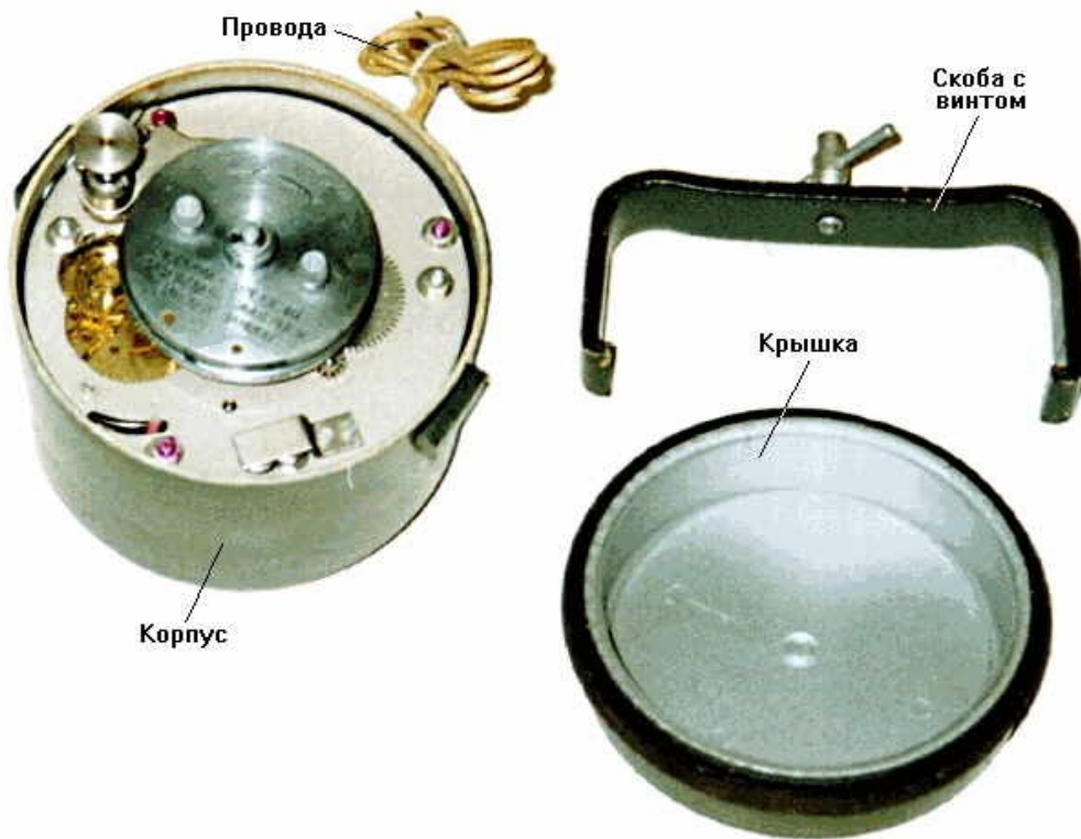
ChMV-120 showing cover and bracket, note the combination tool closing screw
