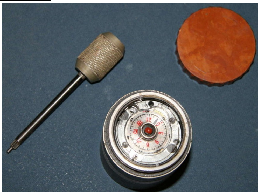
VZD-144Ch with cover off and showing time setting tool.
