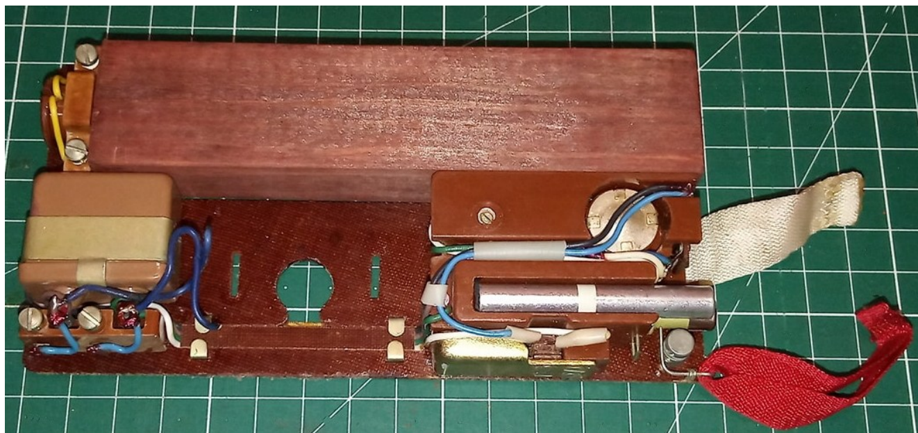
Internals of MS-4, wooden block representing the explosive charge Photo- Oleksandr Mariash
