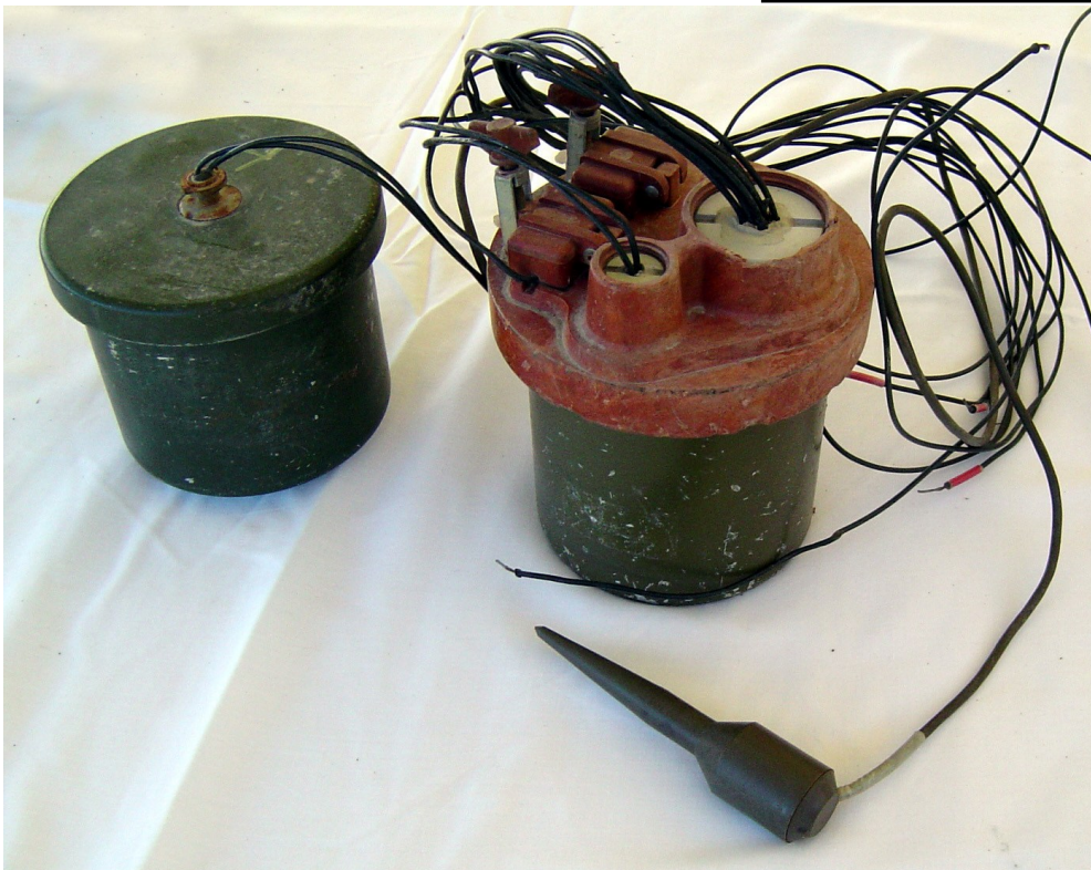
VP-04 Firing Device showing geophone and signal processing device. Photo– C. King
