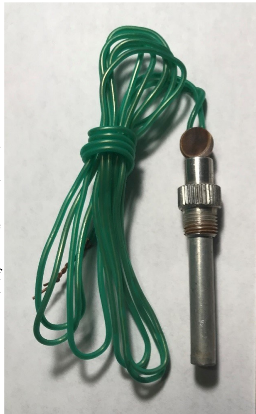
EDPr Detonator Assembly Photo- G. Zahaczewsky
