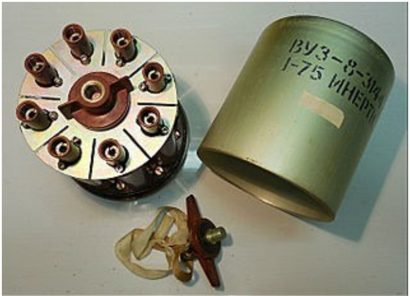
VUZ-8 with cover removed
