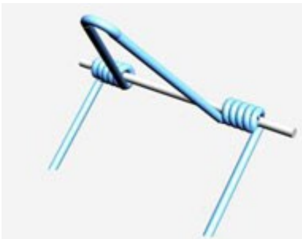
Design of the lift spring for the MS-2
