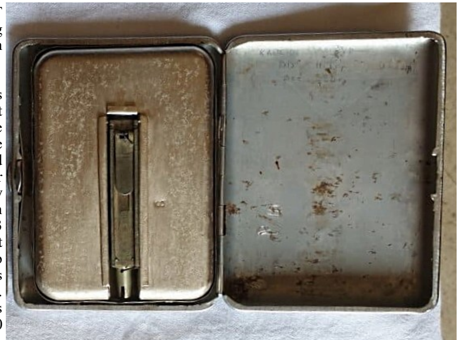
MS-5 Firing device showing the internal mechanism.
