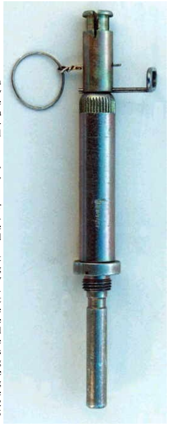
MUV 2 Firing Device Upper safety pin is not as issued
