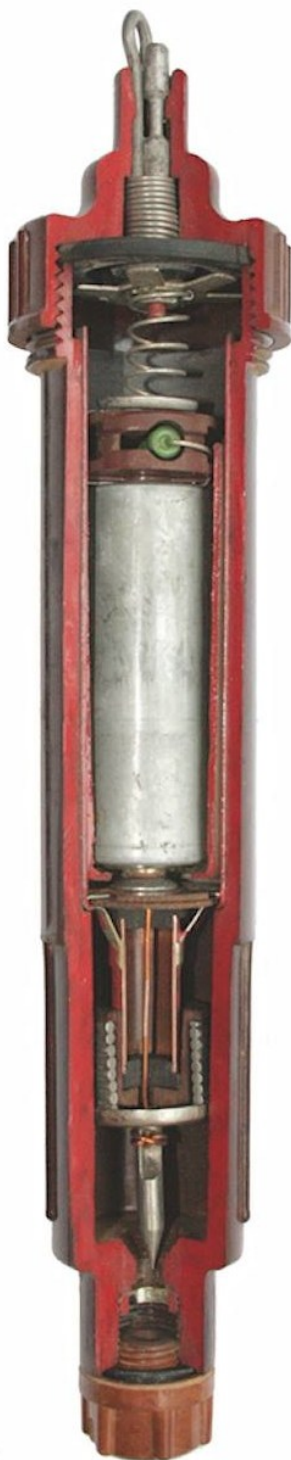
Sectioned EKhV-7 Photo- CAT-UXO
