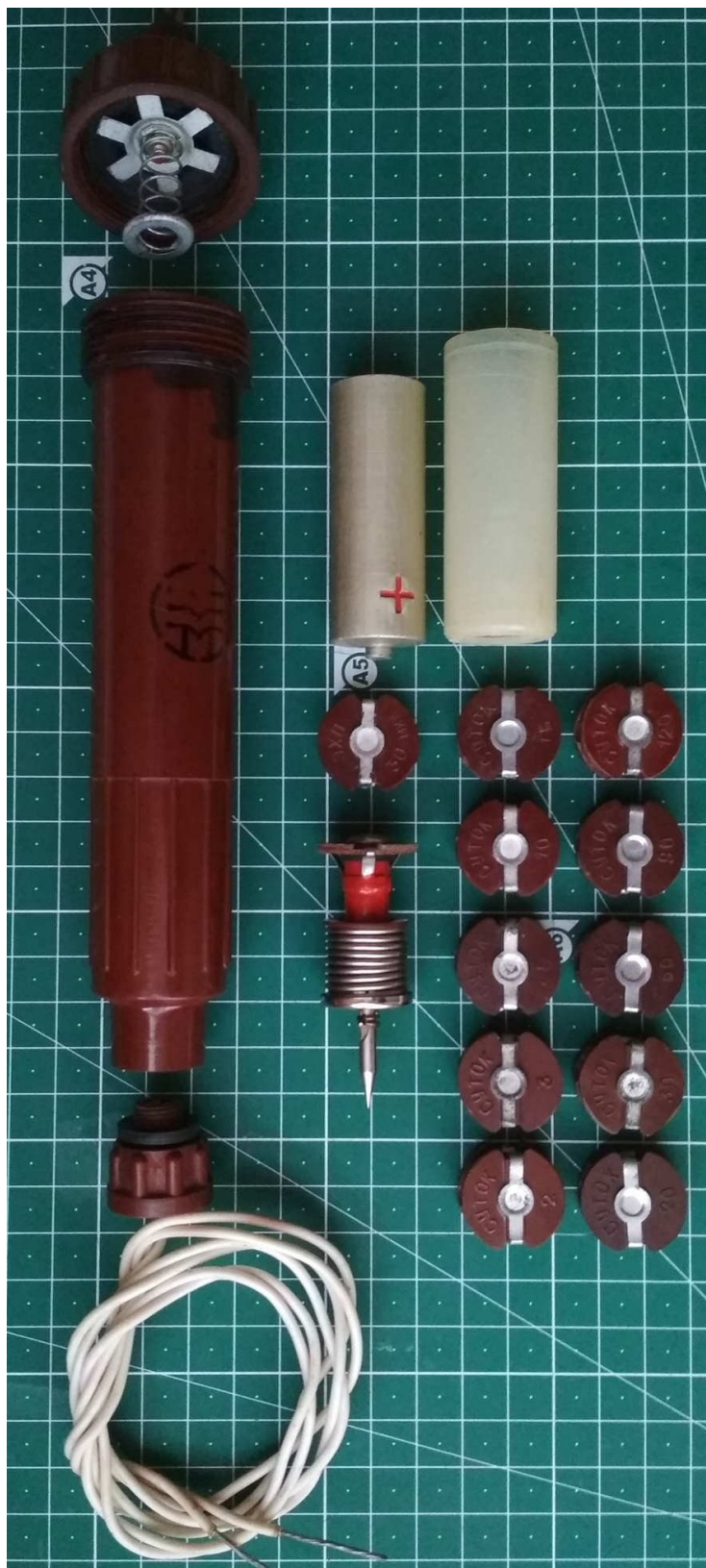
EKhV-7 Firing Device showing internals and a full set of time resistance coils. Note the electrical circuit contact plug.
