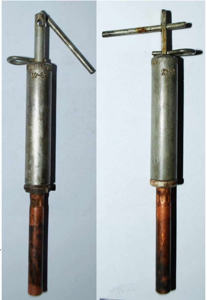
Oval striker MUV on left, flat striker MUV on right
