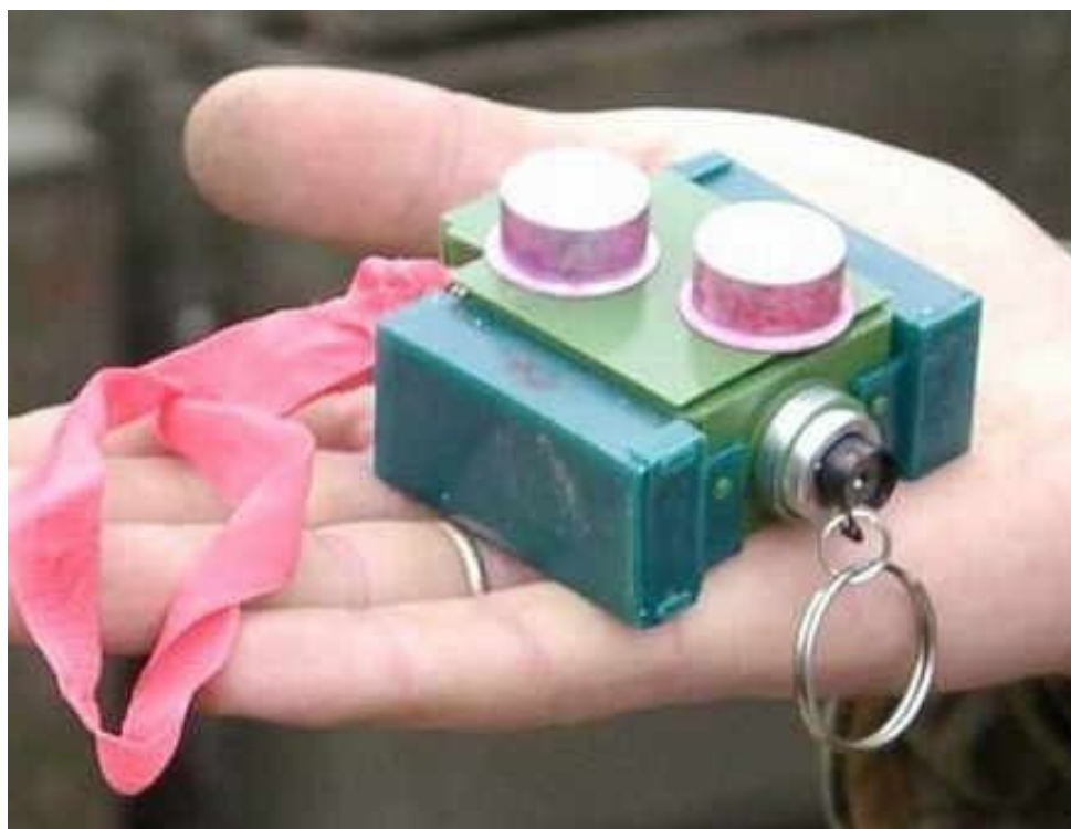
ML-7 Firing Device showing the two removable booster charges
