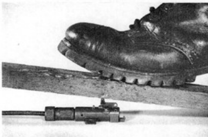
Firing Device, Demolition, F1A1, set for PRESSURE and using safety fuze initiation
