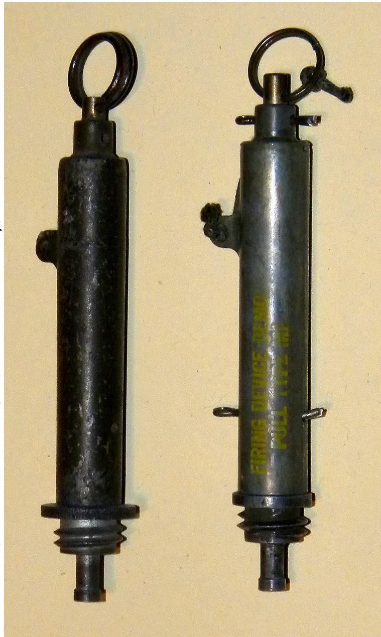
Firing Device, Pull, M1 (New Style) Left- WWII issue, Right- Post War issue
