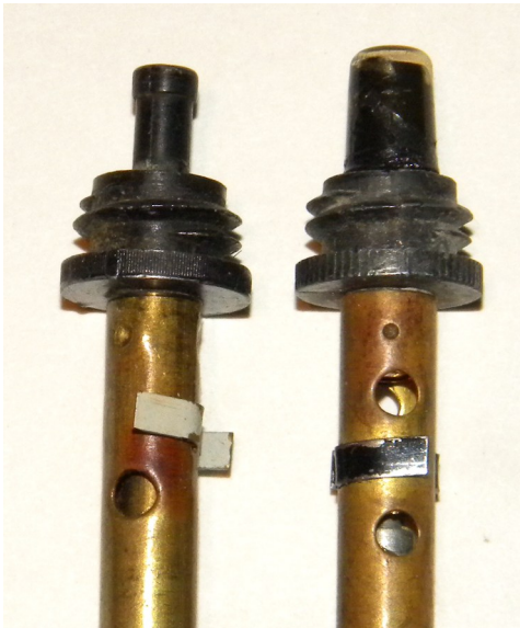
Closer view of the differences in inspection holes.
