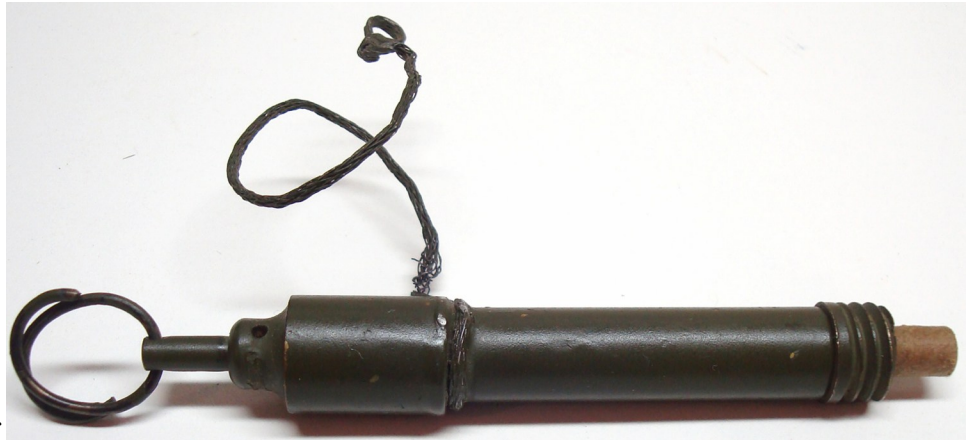
Firing Device, Pull, M1 (Old style) note the anchor wire soldered below the head
