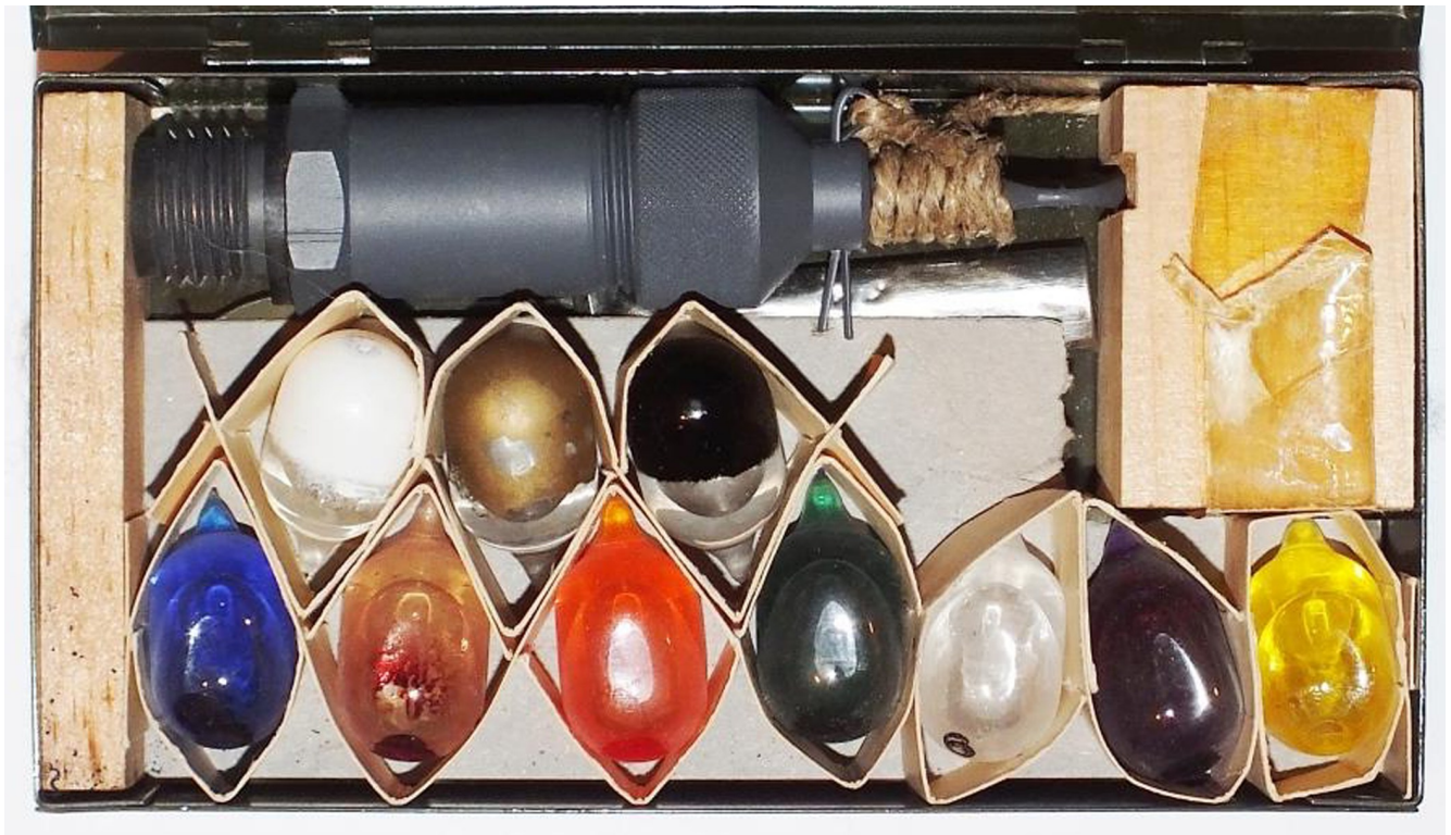
Firing Device, AC Delay, Mk. 1 (early type) in box with 10 ampoules, likely a post war CIA issue.
