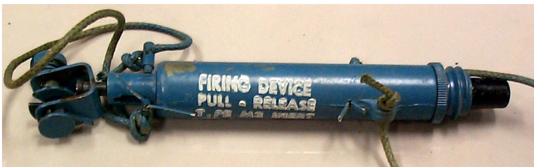
Firing Device, Pull/Release, M3 Inert training device
