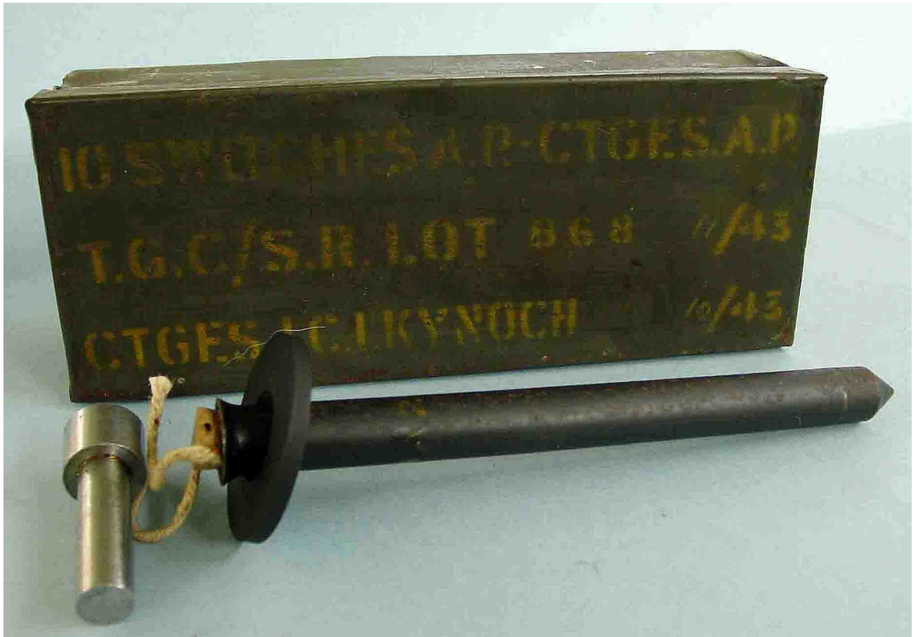
Switch, No. 8, Anti-Personnel, Mk. I with packing box and anvil used for pounding the spike into the ground.
