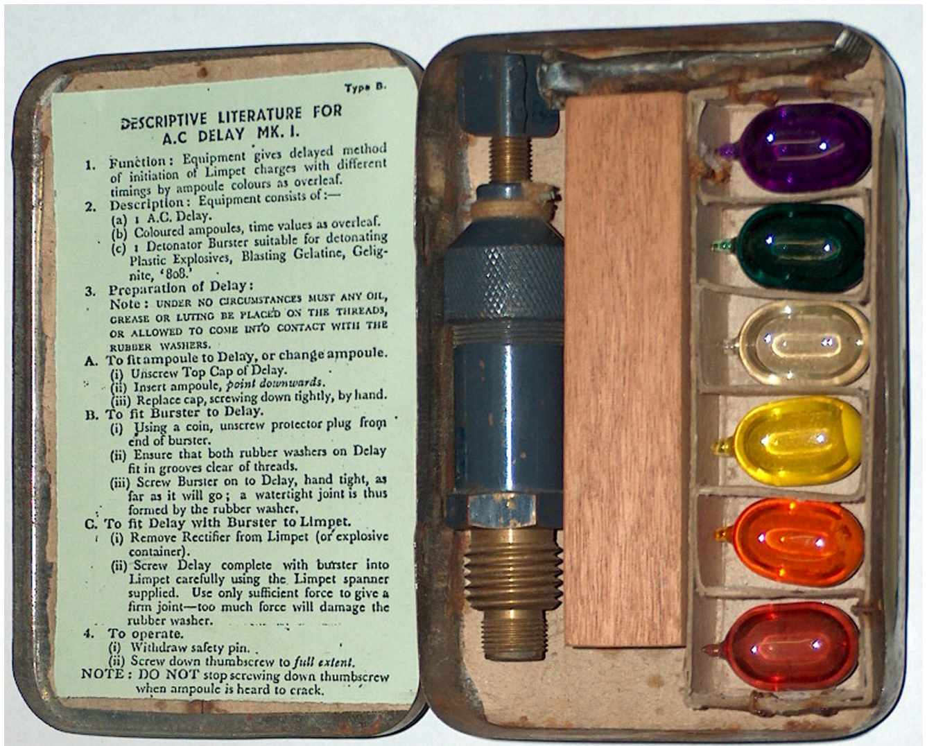
AC Delay, Mk. I in packing box with all parts. The burster is contained in the wooden block.
