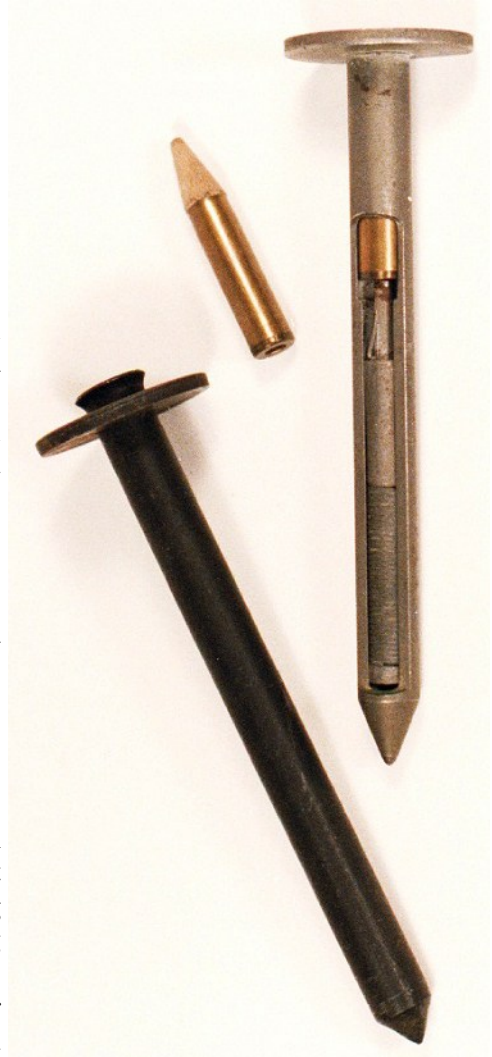
Switch, No. 8, Anti-Personnel, Mk. I Upper Right- early one piece body Lower Left- later version with two piece body
