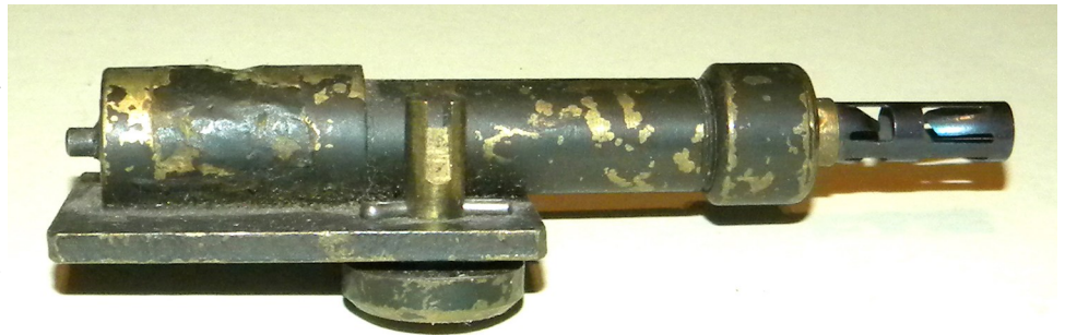
Switch, No. 2 Pressure, Mk. I in stowed position. Note the later spring snout.
