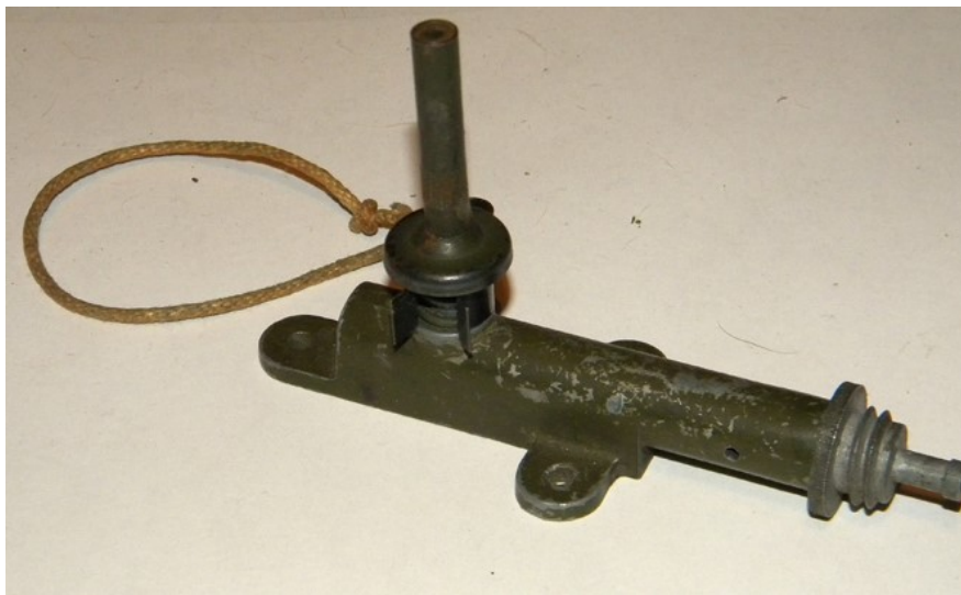
Firing Device, Pressure, M1 (New Type) with extension rod installed
